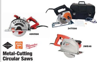
Used in metal fabrication and auto body shops to cut metal when precision is required. They rotate slower and have more torque than general purpose saws to make cleaner, faster cuts. Corded for long run times compared to cordless tools and have no batteries to recharge. **Left Blade Side** makes it easier to see sight lines when the saw is held with the right hand. **Right Blade Side** positions the blade away from the user's body when the saw is held in the right hand.
