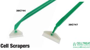
Use for the manual harvesting of cells in tissue culture flasks. ABS handles with TPE blades. Scraper-style blade is positioned parallel to the handle for windshield wiper-like scraping. Lifter-style blade is perpendicular to the handle for use with a raking motion.
