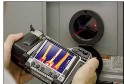
IR windows can be used indoors or outdoors and support Laser LocatIR targeting
