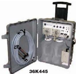
Systems take composite and discrete samples for wastewater, industrial, and environmental applications. Size and interval controls set the individual time-weighted composite samples or full-bottle discrete grab samples. An external-trigger mode controls sampling from a water level sensor, rain sensor, or other external source (not included). Automatic 15-sec. backflush cycle clears debris from the strainer and empties water from the hose to prevent contaminating the next sample.
