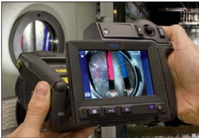
Visible light is clearly transmitted to capture visual as well as infrared images (LED lamps recommended)
