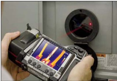
IR windows can be used indoors or outdoors and support Laser LocatIR targeting
