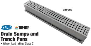
Compatible with various pipe sizes including 4" dia pipe. Drain Sumps with **Grate** feature a universal snap-in pipe seal and a contoured bottom that directs all water to the drain to help eliminate standing water. For use in landscape or hardscape drainage and below downspouts. Trench Pan Drain and Trench Pans are for use in concrete, linear surfaces including driveways, floors, and truck docks.
