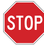
R1-1 D9768 HIP (12 in x 12 in, 18 in x 18 in, 24 in x 24 in, 36 in x 36 in) D (12 in x 12 in, 18 in x 18 in, 24 in x 24 in, 30 in x 30 in, 36 in x 36 in)
