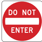
R5-1 D9624 D, HIP (24 in x 24 in, 30 in x 30 in) HIP (12 in x 12 in)
