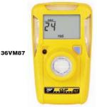
Compact, lightweight design features 1-button operation and 2 yr. continuous use without calibration, sensor replacement, or battery recharging/replacement. Extend the working life of detectors with the Hibernation Case, sold separately.
