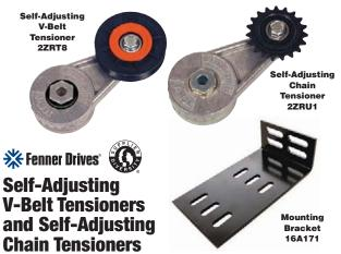
Spring-loaded to maintain correct tension on belt and chain drives without requiring manual retensioning. Models having **Accurately Wound Compression Springs** provide a constant retensioning force. **Torsional Wrapped Spring** models feature a reversible spring for bidirectional use.
