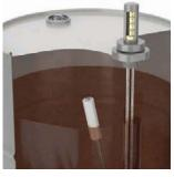
Gauges have stems with extended arms that have a floating component that moves up and down as the liquid level changes to measure fluid levels. They install on the tops of vertical drums and tanks and provide continuous, reliable measurements without requiring a power source.
