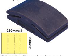
Suitable for all types of coated abrasive sheets. Accepts a standard 230  $\times$  280mm sheet split down into quarters across the width, as shown.
