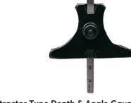
Protractor Type Depth & Angle Gauge Ground steel with graduations from 0° - 180° in both directions. When rule is positioned to 90° it then provides accurate measurements of depth.
