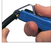
For stripping of all common round cables of 4 - 28mm. Wire stripper adjusts automatically to diameter of wire to allow quick and accurate stripping. Stripping blades are made from hardened steel.
